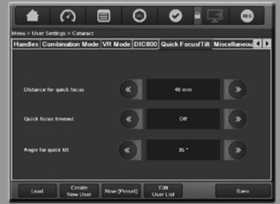
Select Quick Focus to immediately switch between two different focal planes and Quick Tilt for workflow efficiency in glaucoma procedures
