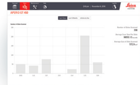
Stats page allows you to view slides scanned/day/month/year, average scan area and average scan speed.
